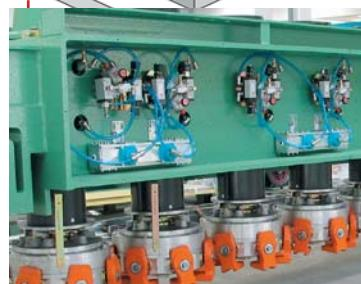
Modular distribution manifolds on machines or automatic lines.
