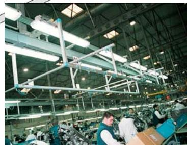
Workbenches for assembly operated with pneumatic and electrical tools.
