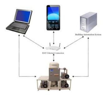
PBMI – our "Powerex Building Management Integrator" was designed specifically for medical facilities that have a Building Automation System (BAS). Our PBMI is a communication gateway utilizing BacNet® protocol. It features pre-configured and labeled data points along with email notification. This truly is a "plug and play" integrator that allows our medical systems to easily communicate with the facilities BAS, keeping you in touch with your facilities Powerex equipment no matter where you are.
